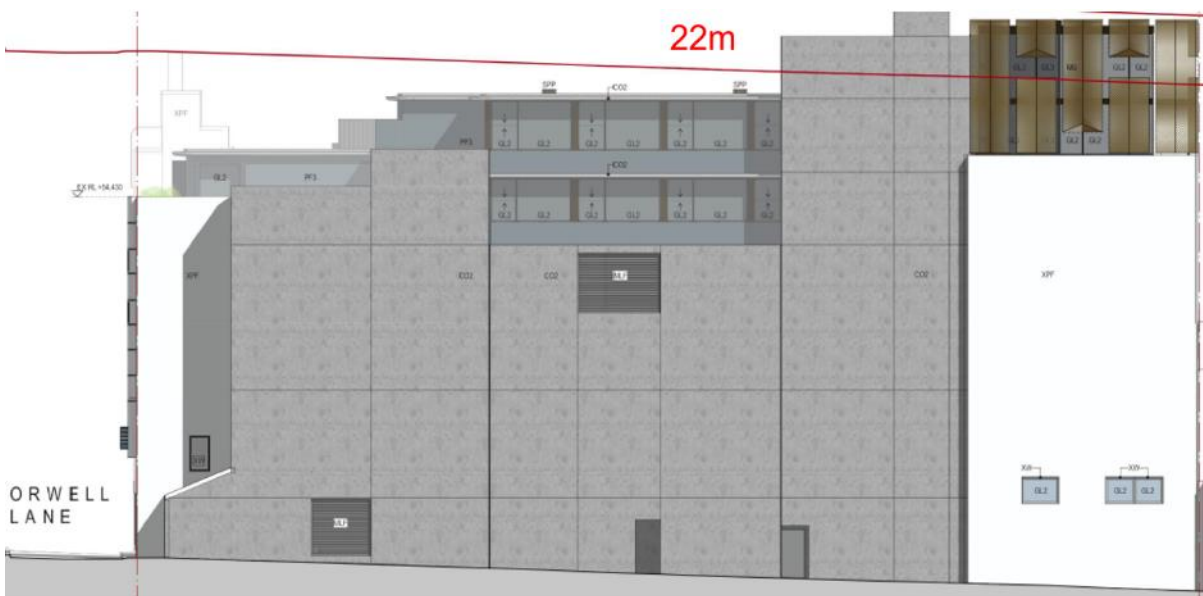
Figure 44: The height limit (shown as a red line) as viewed from the northern elevation
